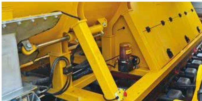
18. A hydraulic piston able to regulate, with shutters, the flow independently according to the casting needs
