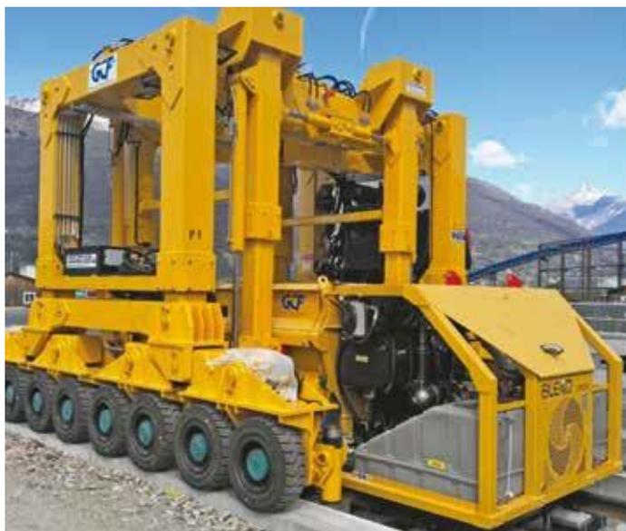
14. The mobile portal crane wagon and the mixer for speeding up the casting operations in the tunnel
