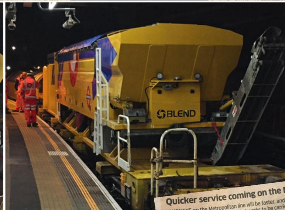
Safety is guaranteed using barriers (chains and doors) on board, fire extinguishers and signal lights that warn about plant passage in the tunnel.
