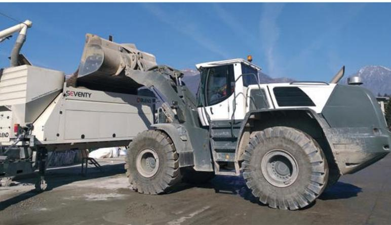
Feeding recycled aggregates into the loading hoppers using a 4m<sup>3</sup> wheel loader.
