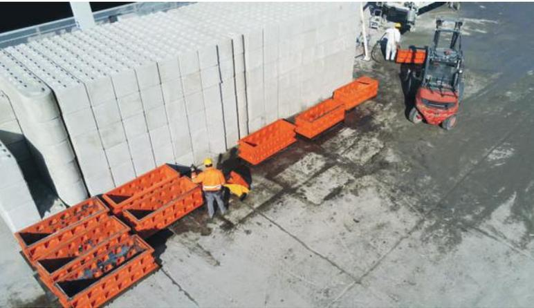
The Betonblock elements are produced using 20 molds. Their modularity allows to produce also elements with rounded profiles for irregular angles.
