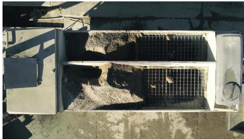
The loading hoppers for the aggregates are divided in a rational way, making loading easy with a wheel loader.
