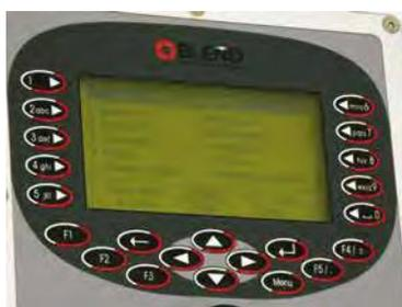
9. The command display, which is perfectly watertight, allows simple insertion of recipes and working functions. A remote control allows the plant to be operated from remote.
