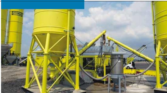
7. Additive mixing is possible by adding other types of external supply to the hoppers on the machine
