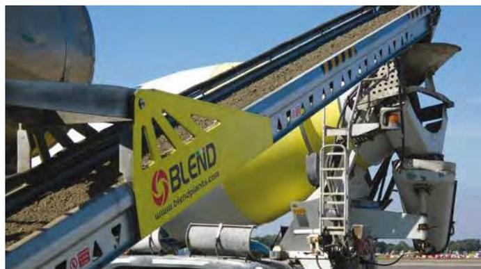
10. Loading the cement lorry is direct using the remote controlled belt that speeds up operations
