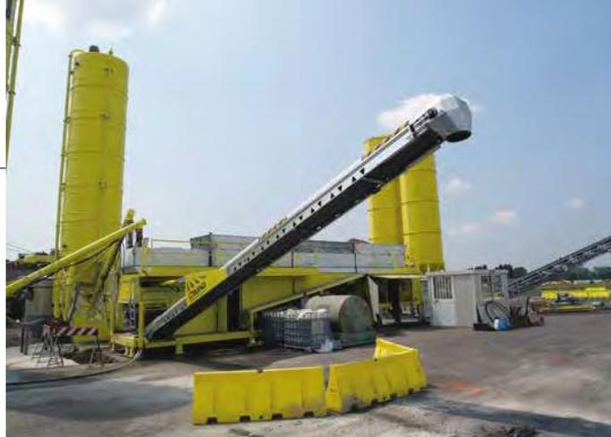
8. The Blend A240 was positioned near a plant for cement mixes only which, in production peaks, was assisted by the Brescia-manufactured machine. The functionality of this A240 was particularly appreciated on the building site allowing quick changeover from cement mixes to specific RCK
