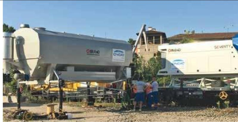
10. The combination of plants assembled on rolling stock and horizontal silos further increases working efficiency and speeds up operations and improves autonomy.
