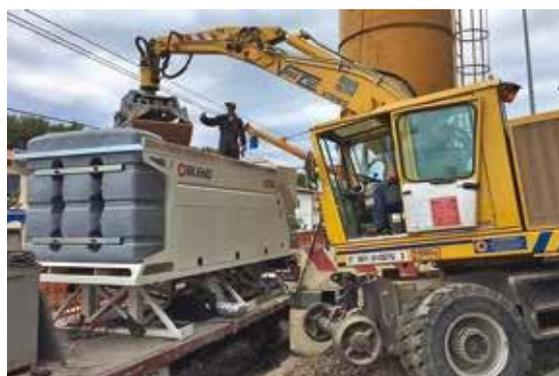
4. Aggregates are quickly loaded both with rail loaders and using other belt or hopper systems, demonstrating ample adaptation to any operating situation.
