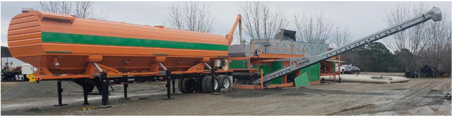
7a-7b. The A240 plant with the horizontal silo, purchased from TCP Concrete, worked day and night, producing about 20,000 m<sup>3</sup> of concrete.
