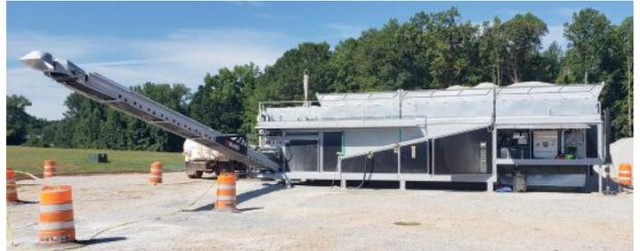
9. The A240 plant used by Robert Smith Inc. produced 14,000 m<sup>3</sup> of RCC concrete in just two and a half months.
