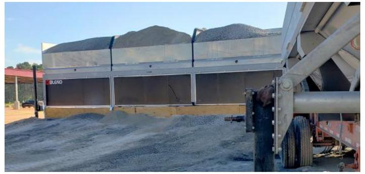
**5.** A240 is available with 2, 3 or 4 hoppers. The reduced height of the plant means that loading of the aggregate hoppers using a wheel loader virtually eliminates the need for a ramp.
