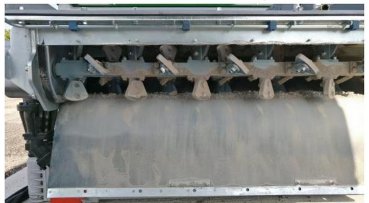
**6.** The continuous twin shaft paddle mixer slides out on rails to facilitate cleaning and maintenance.
