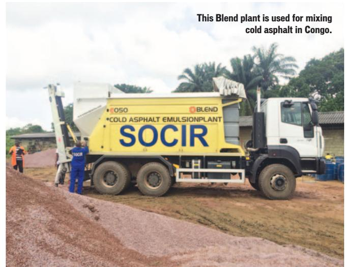
This Blend plant is used for mixing cold asphalt in Congo.
