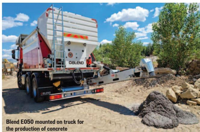
Blend E050 mounted on truck for the production of concrete
