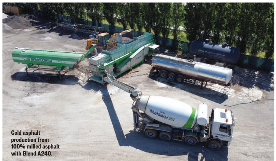
Cold asphalt production from 100% milled asphalt with Blend A240.
